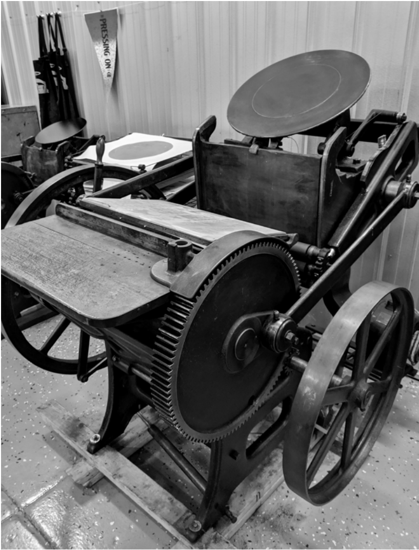
Fig. 1.1. 12 × 18 c&p platen press from Tribune Showprint, Muncie, Indiana. Photograph by Kathy Ferguson. Courtesy of Rob and Kim Miller.
