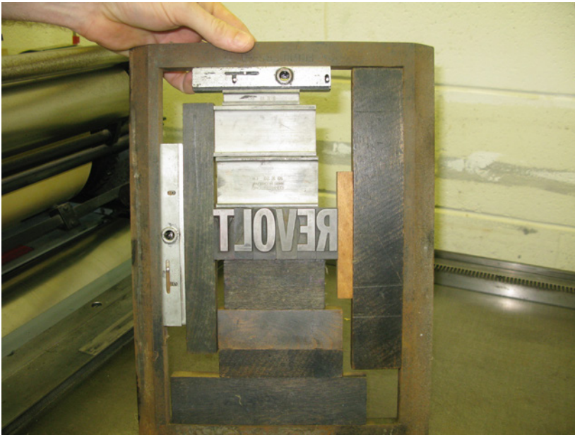
Fig. 1.5. Chase locked up as shown by Duncan Dempster, University of Hawai‘i. Photograph by Kathy Ferguson.
